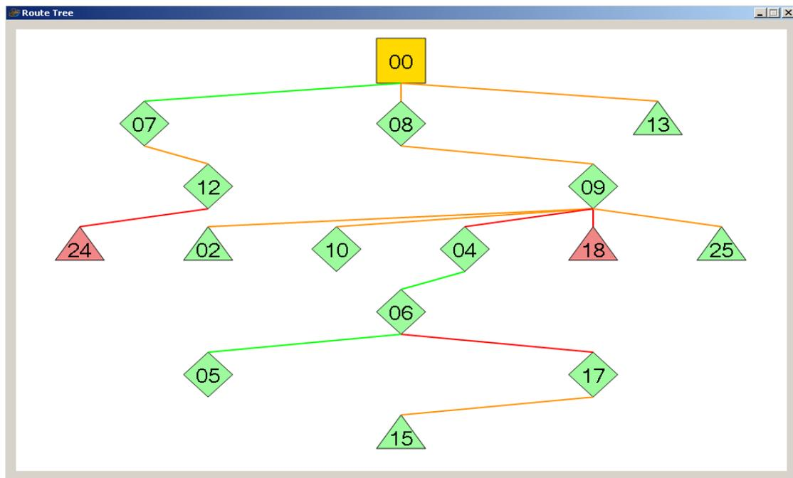
5. **NOTE: Only mains powered nodes can assume a parent role!** A parent must be always awake waiting for data! This is not possible for battery powered nodes; these sleep most of the time and can not stay awake as their battery will be fast exhausted
